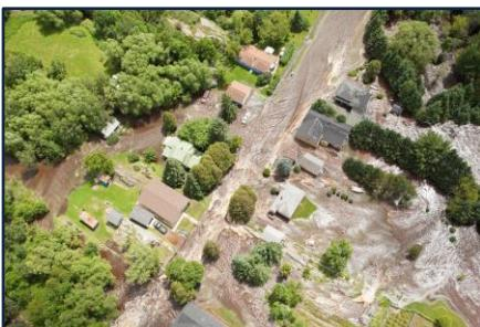
Floodways are critical parts of floodplains that communities need to take particular care to manage well. Floodways see the fastest moving and deepest floodwaters, making them the most dangerous places for buildings, infrastructure, and places for people to go. They also typically host the most beneficial ecological functions of floodplains.
