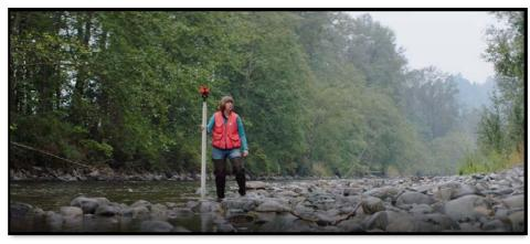
Patty Dillon, principal hydrologist, surveys the Snoqualmie River in Washington State to identify changes in slope to get the overall shape of the river, which informs the creation of flood maps.
