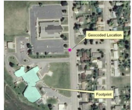
Example of a geocode point and building footprint of a county building
